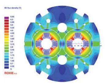
ROXIE simulation of the field in the magnetic yoke of MQY, one of the LHC matching section twin aperture quadrupole magnets. (Glyn Kirby, CERN)
