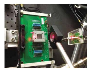
Experimental set-up in CERN building 27 to test the depth of interaction capability for LYSO crystals coupled to a SiPM. (CERN/CrystalClear)
