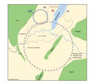
Schematic of an 80-100 km long circular tunnel for the FCC. (OPEN-PHO-CHART-2014-003-1)
